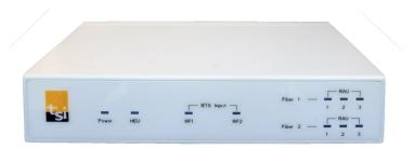
The sDAS system includes the HEU and RAU. The HEU can take RF signal from any source like Macro/Pico/Repeater/Small Cell and distribute the signal to RAUs in different locations via the single fiber. Each HEU can convert and distribute the RF signal to max. six RAUs to 5km distance. Both star and daisy chain topology are supported
