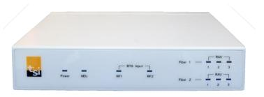
A sDAS system includes the HEU and RAU. The HEU can take RF signal from any source like Macro/Pico/Repeater/Small Cell and distribute the signal to RAUs in different locations via the single fiber. Each HEU can convert and distribute the RF signal to max. six RAUs to 5km distance. Both star and daisy chain topology are supported
